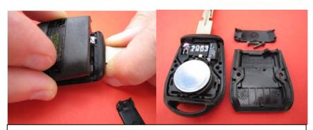
Lift back cover to uncover electronic board with immediately visible battery. After opening you will end up with parts as pictured above.
