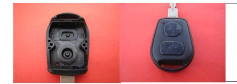
Once your silicone buttons are fitted in, place electronic board back in remote (after removing rubber band), cover it with bottom part of the shell and screw screws in using pozidriv driver. **No reprogramming is need it** as remote will work straight away.
