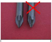
**Do Not use Phillips screwdriver** (shown on the right) as you may damage screws
