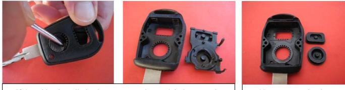
If the rubber is well glued you may need to push it down gently from the top. For easier removal, hardened rubber can be softened with a hair drier set on low heat. You should end up with cover looking like one in the picture above, free from old rubber remains Now you can simply press fit Silicone repair buttons from outside of the shell.
