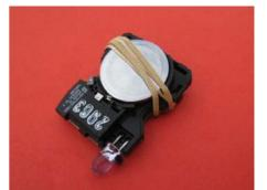
When you come to lifting electronic board you would have to put battery aside as it will not stay on board. **In most cases you have up to 60 sec before your remote may lose memory** (check your user manual)
