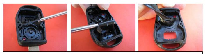
Use flat screwdriver to lift up old rubber pad. Do it gently so you do not damage hard shell. Once rubber starts parting from plastic cover, start pulling it gently and detach it.
